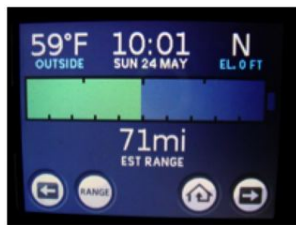
Sample of battery ½ depleted.
